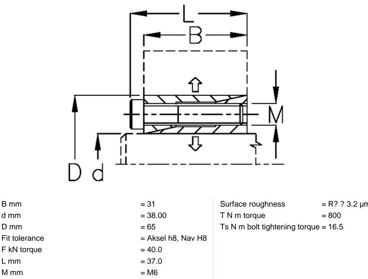
P N/mm2 surface pressure on shaft/hub = 90
